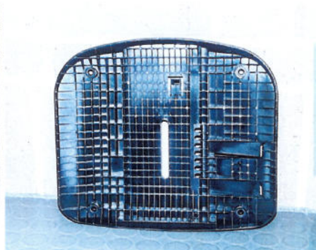
Photo 1 Test set up / Photo 2 Seat shell after 315 400 cycles / Photo 3 Seat plate made of Polypropylene
